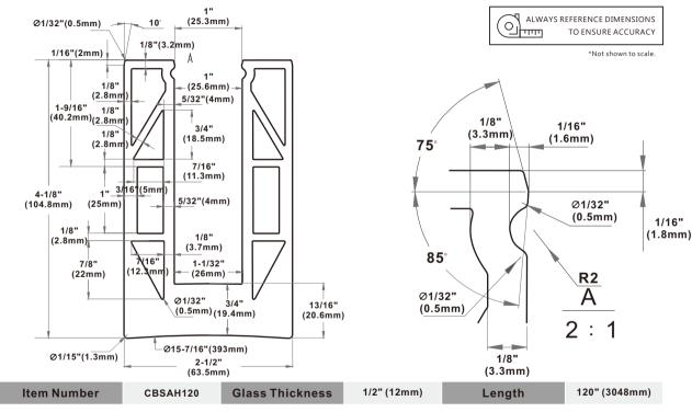
Heavy Duty Glaze Commercial Base Shoe 120" Length, Drilled For 1/2" Glass
